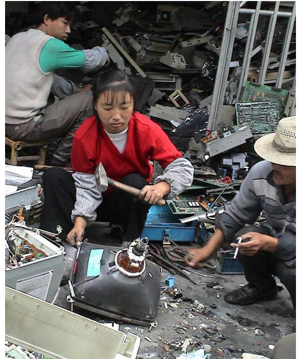
Woman in Guiyu, China, about to smash a monitor, to remove the copper yoke at the end of the funnel. The glass is laden with lead, but the biggest hazard from this is the inhalation of highly toxic phosphor dust coating inside. December 2001. Copyright: Basel Action Network.
